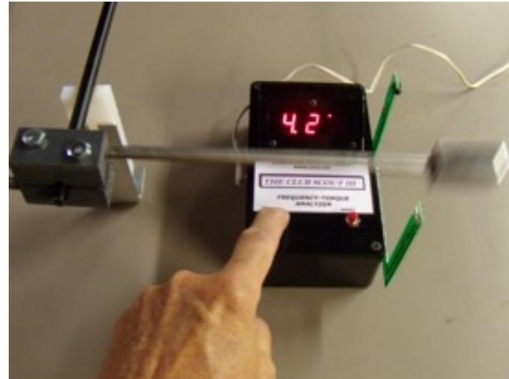
corner of the box contains a window with a IR light source and a phototransistor. The transistor senses the reflection of the IR beam off of the shaft. For non reflective shafts a small piece of reflective tape must be attached to shaft to get a reflection. The Jr.CS is more sensitive to outside IR light source so caution is advised. The on/off switch doubles as a reset switch.
