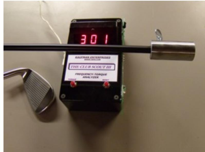
alignment is a bit below the sensors. The grip will result in dampening and lower the frequency by about 5 to 7 cpm.
