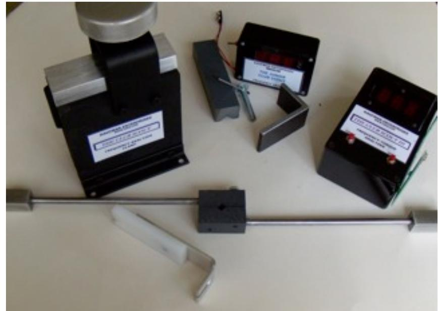
floating V block which is placed on the top of the shaft. An upper U shaped bracket contains a slip clutch which applies the force to clamp the shaft between the two V blocks. When tightened, the clutch will slip with about 300 pounds of force on the shaft. To provide accurate readings the Clamping unit must be firmly mounted to a work bench and the bench itself must be reasonably solid. A loose clamp or wobbling of the bench will lower the frequency by one or two
